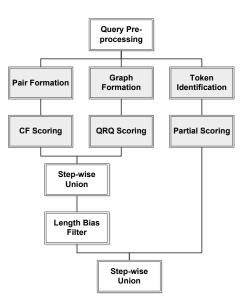
Figure 4: Dataflow in the Metaphor pipeline. Each stage consists of one or more MapReduce jobs that process loaded query and click data.
