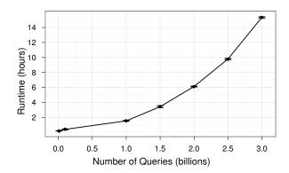
Figure 9: Runtime of the Metaphor pipeline while varying the size of the input query log. The pipeline was run on a dedicated 80-node Hadoop test cluster for 5 trials each.
